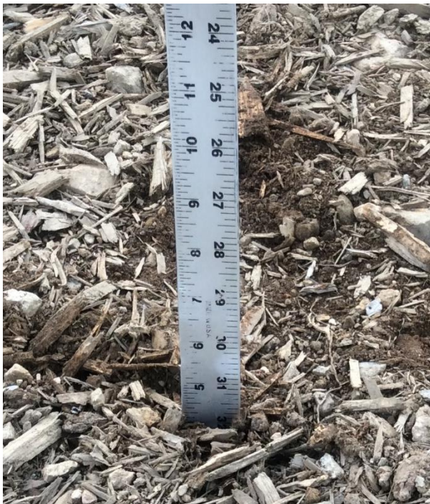
Figure 2: Soil depths were checked at random points on all Pads. They were also coordinated with having wood chips or Jute Mat. This is a 4-inch soil depth with wood chips.
