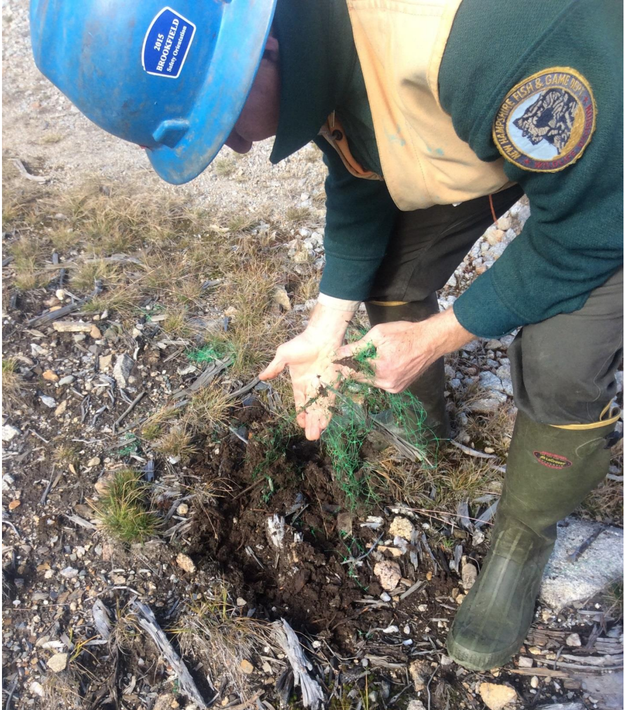
Figure 13: Green erosion mesh. This was picked up from soil removed from roadside, and was then still in the soil on pads after re soiling the pads.
