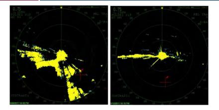
**Figure 2-2.** Screenshots from actual radar files showing ground clutter in horizontal mode (left) and vertical mode (right). Although the radar records three-dimensional space, it is translated by the radar screen as a two dimensional representation, which can cause targets to be obscured from view.
