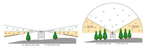
**Figure 2-3.** An example of a tree of a specific height that causes ground clutter, but "masks" a section of the radar beam, allowing adequate detection of targets beyond it (left). The effect of ground clutter on target detection in vertical mode is also shown (right).
