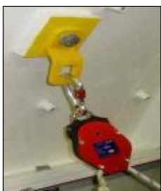
Secure equipment in certified anchor points.
