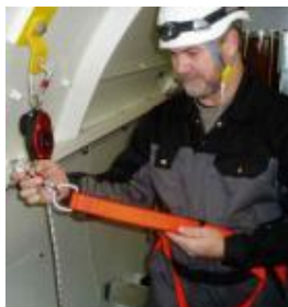
Anchor harness in evacuation equipment
