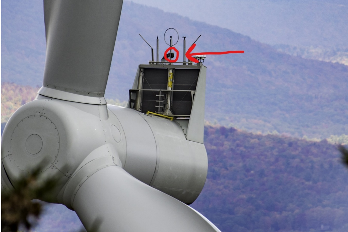
Figure 2-1. Close-Up of a Wind Turbine with an Acoustic Bat Monitor Mounted at the Back End of the Nacelle
