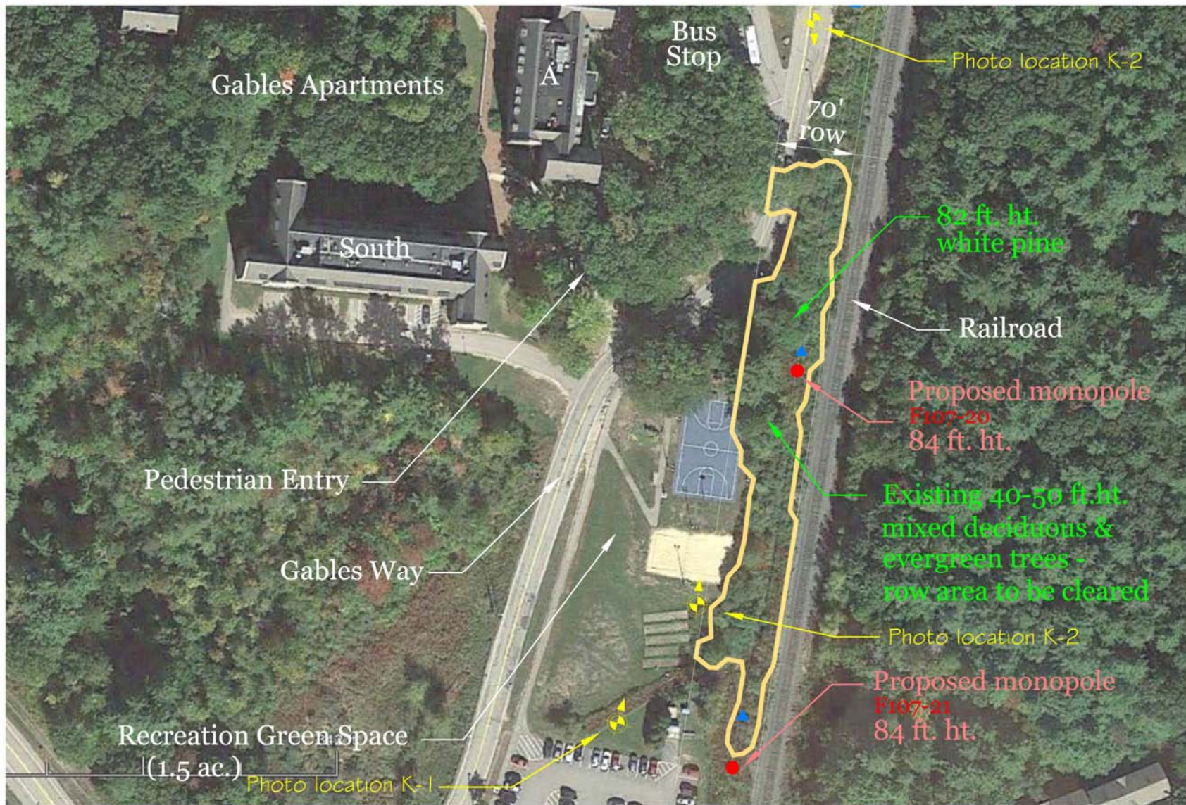
NH Seacoast Reliability Project - Aesthetic Analysis Review K. UNH - Gables Apartment Complex - Main Entry Clearing diagram with tree and pole heights
