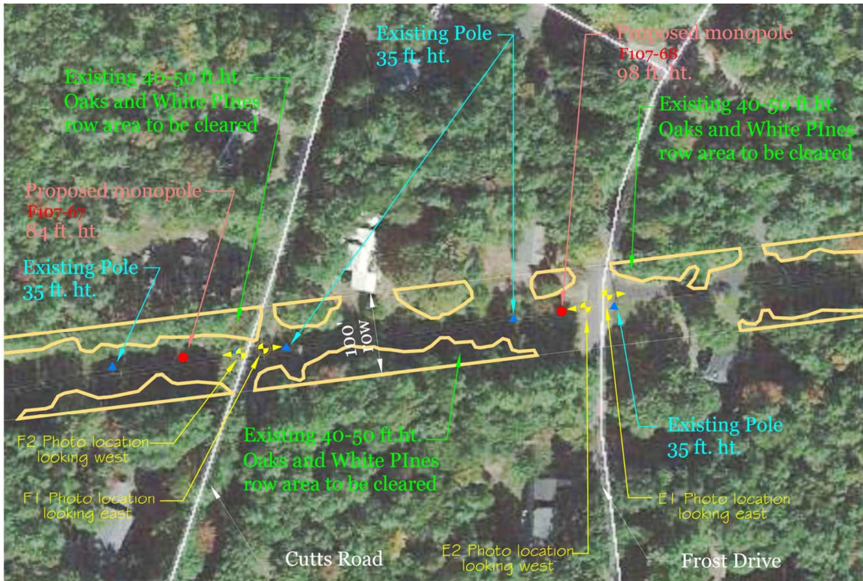
NH Seacoast Reliability Project - Aesthetic Analysis Review E. Frost Drive Crossing & F. Cutts Road Crossing Clearing diagram with tree and pole heights
