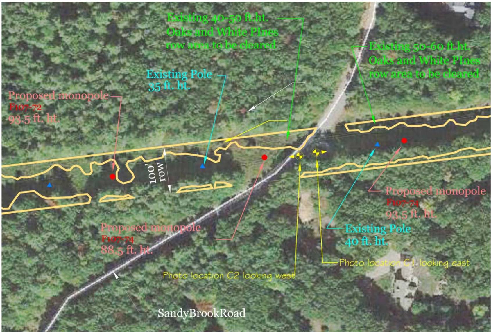
NH Seacoast Reliability Project - Aesthetic Analysis Review C. Sandy Brook Road (east) Crossing Clearing diagram with tree and pole heights
