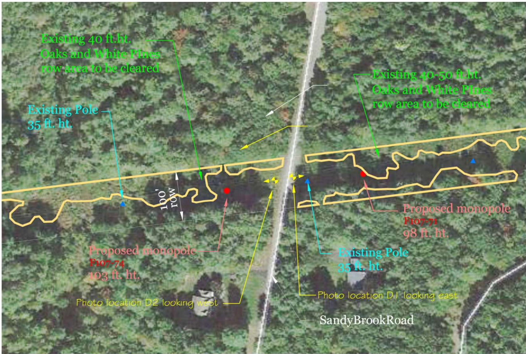
NH Seacoast Reliability Project - Aesthetic Analysis Review D. Sandy Brook Road (west) Crossing Clearing diagram with tree and pole heights
