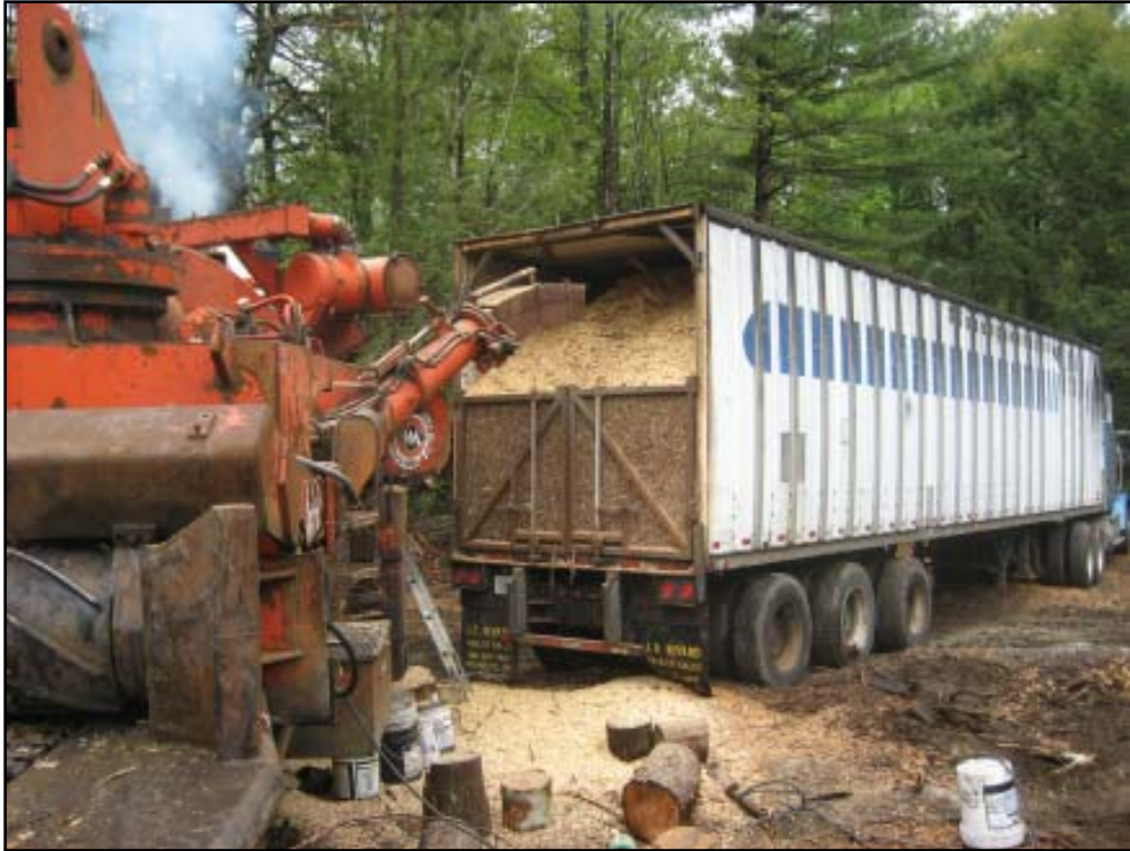
Figure 5. Trailer for whole-tree chips, with opening for chipper to blow chips into.
