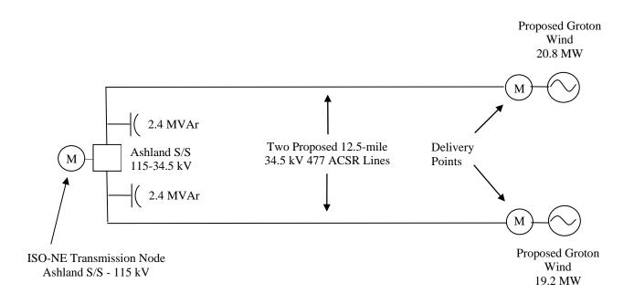
Figure 3: System Configuration for Option 3
