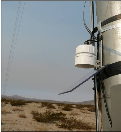
Figure 2: Anabat and “Bat Hat” Installed at Dillon Wind Project, CA
