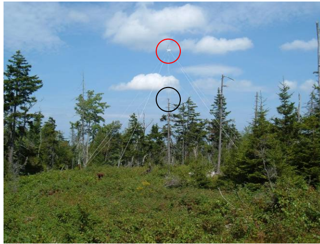
Photo 3-1. Braley Hill Detector. The red circle shows the location of the detector on the portable tower and the black circle shows the tree top location of the detector after the tower collapsed.
