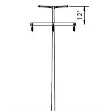
STRUCTURE 138 SINGLE POLE TYPE SS-H-FRAME
