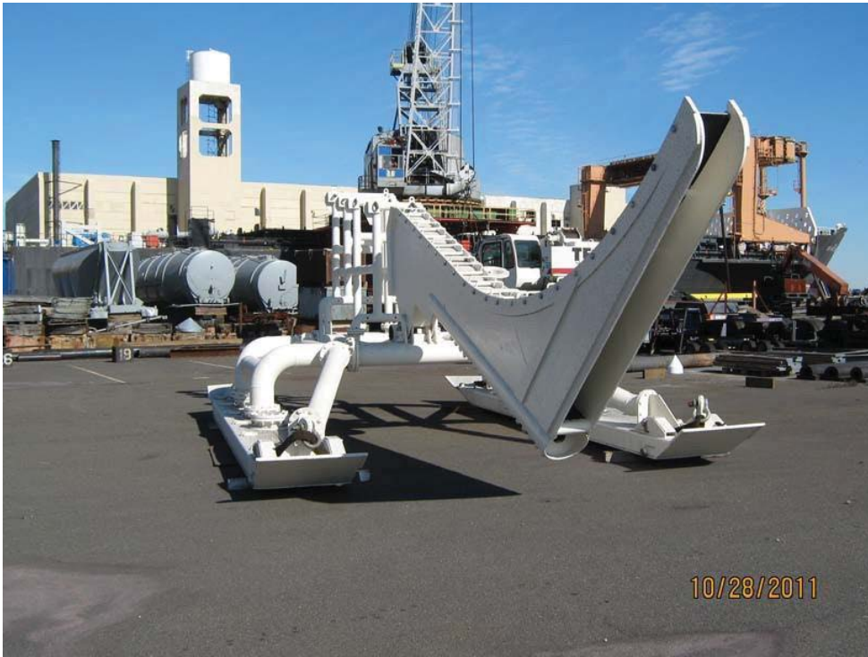
Photo of cable jetting sled (left side-back)
