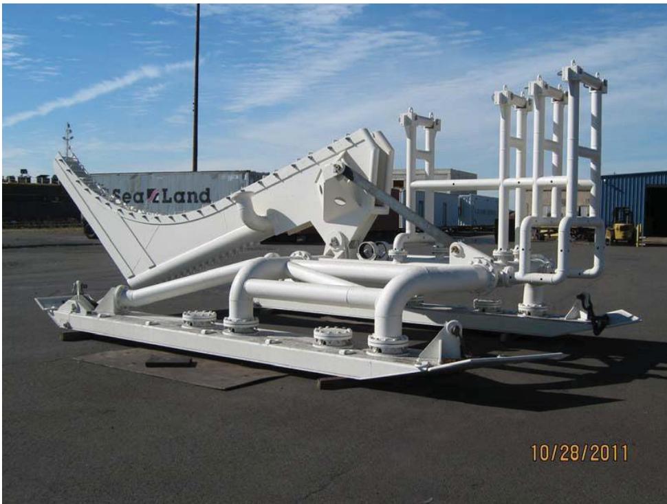
Photo of cable jetting sled (right side-front)
