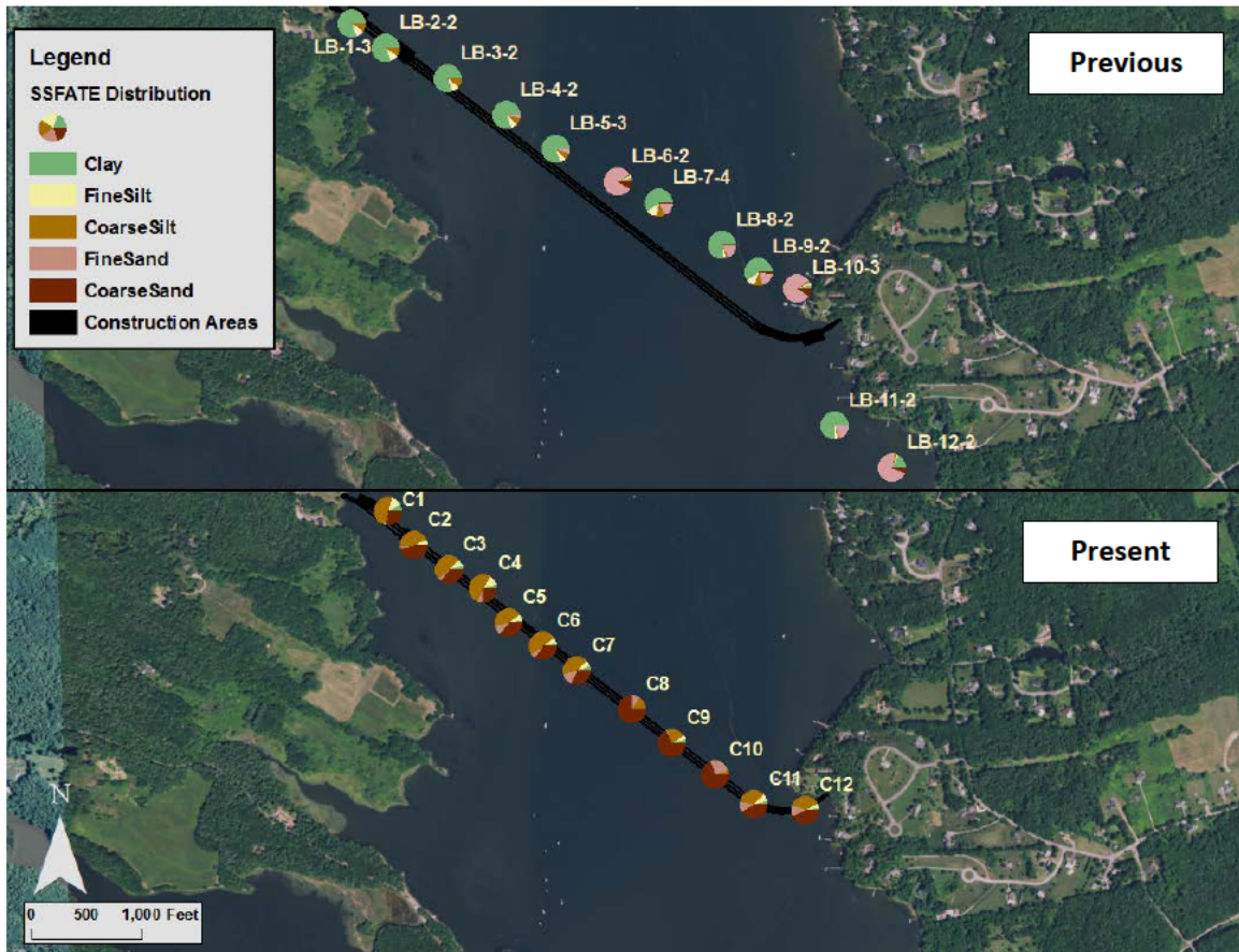
Figure 1-4. Illustration of previous (top) vs. present (bottom) grain size distribution delineated in classes used by the sediment dispersion model.
