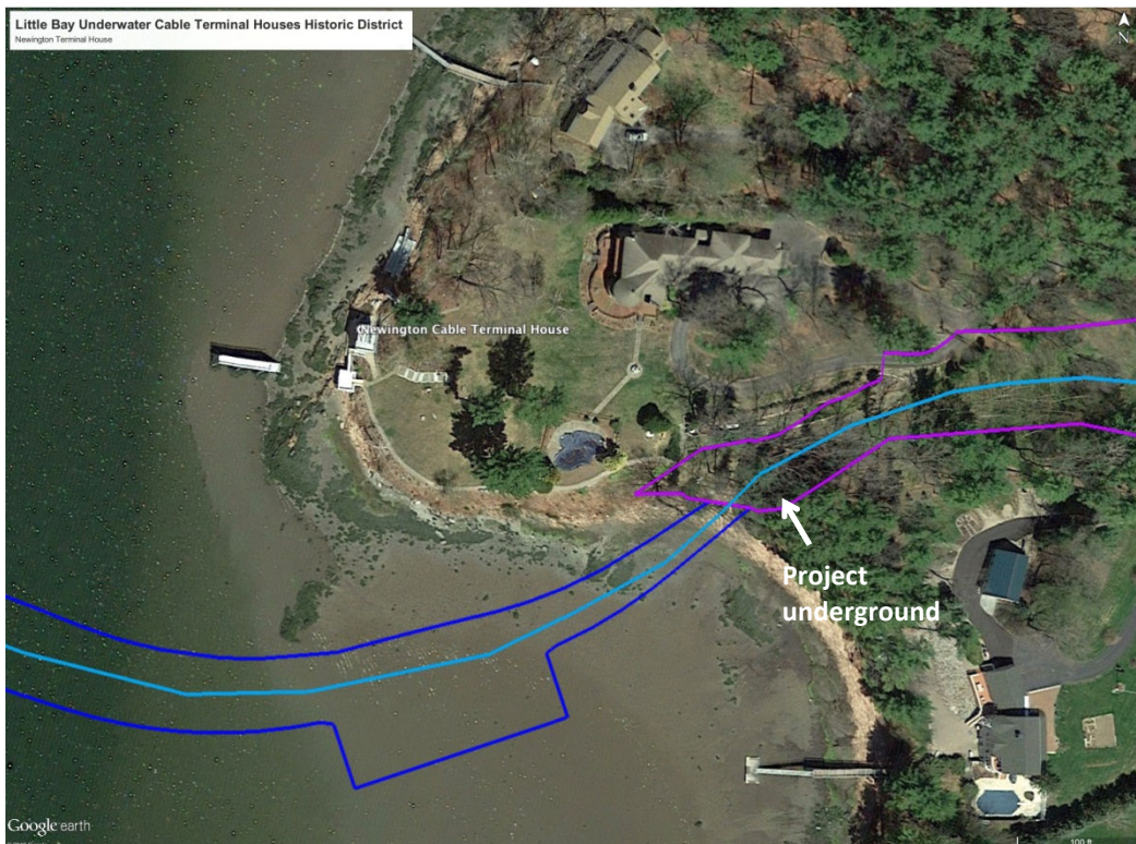
Satellite image from Google Earth of the Newington Cable Terminal House location, showing the proposed project above ground and the location of the underground (blue line), right of way (purple lines) and submarine right of way (dark blue lines).
