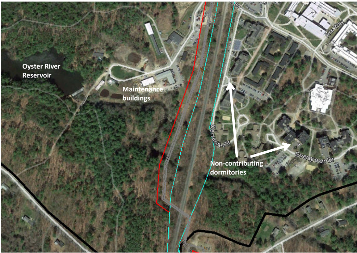
Proposed overhead in electric utility right of way (red line) west of railroad corridor (blue lines), between new dorms and modern maintenance facilities
