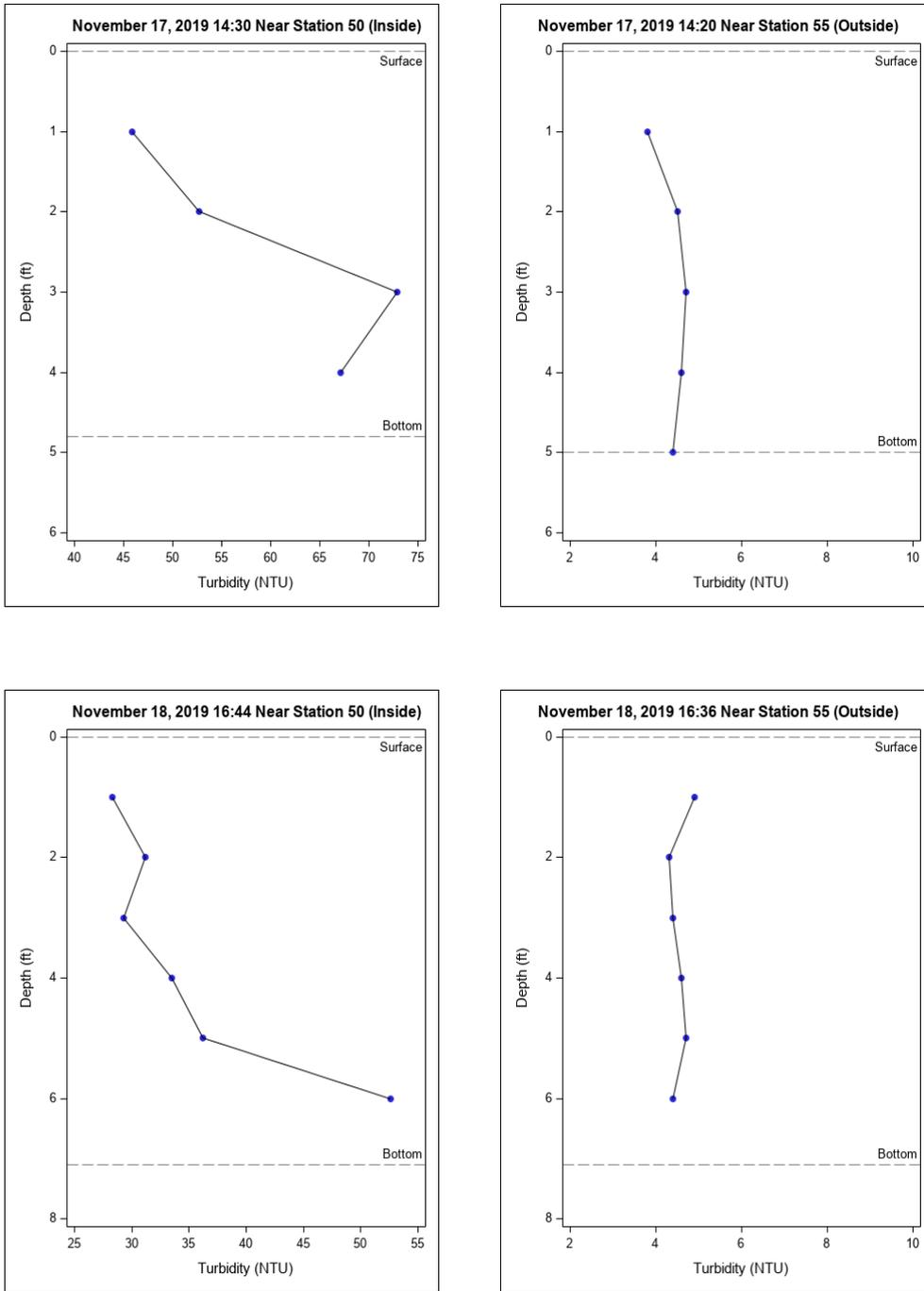
**Figure 2. Vertical profiles comparing turbidity levels within the turbidity barrier, and adjacent to and outside of the barrier.**
