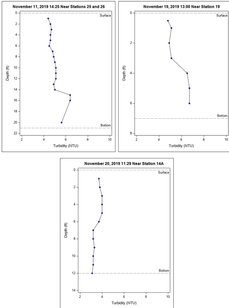
**Figure 1. Turbidity profiles for three plumes identified during hand jetting in the east channel (no turbidity barrier).**
