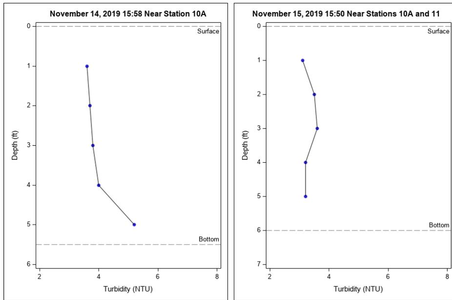
**Figure 3. Turbidity profiles for two plumes identified during hand jetting in the western tidal flat (with turbidity barrier).**
