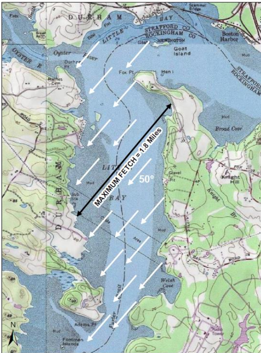
Figure 1. Wind fetch in Little Bay for wind direction of 50 degrees (clockwise from true North)
