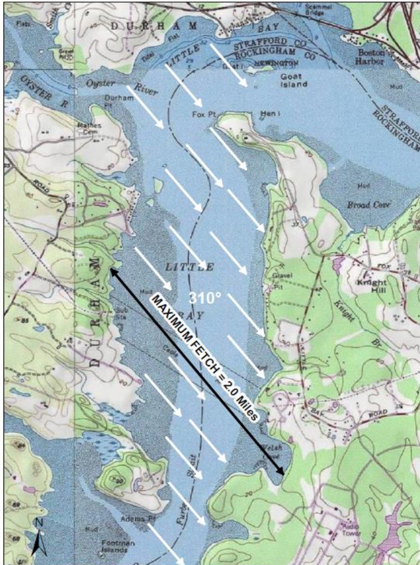
Figure 2. Wind fetch in Little Bay for wind direction of 310 degrees (clockwise from true North)
