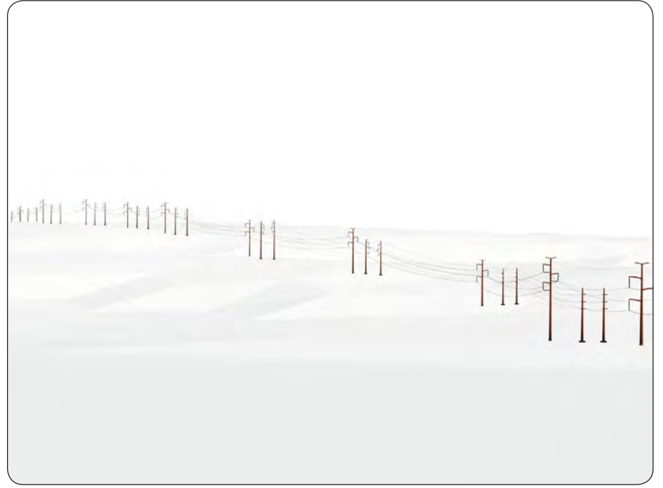
A three-dimensional computer model of the project is built based on proposed structure specifications and structure site coordinates.
