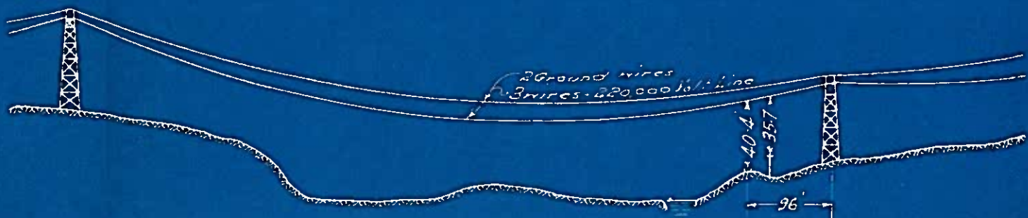
PROFILE OF RIGHT CIRCUIT Scales: Hor. 1" = 160 ft. Ver. 1" = 80 ft.
