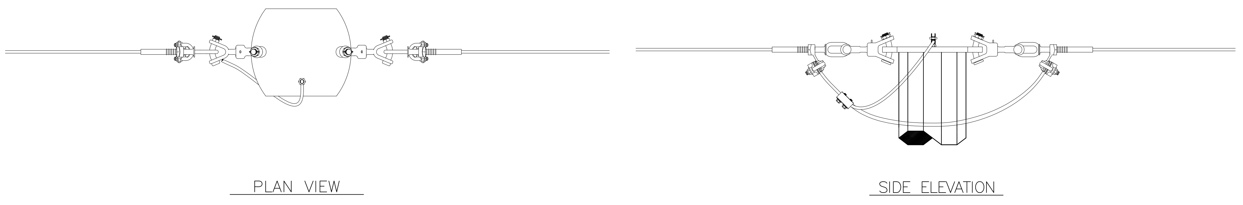
DETAIL 1 SHIELD WIRE ASSEMBLY (TYPICAL 2 PLACES)
