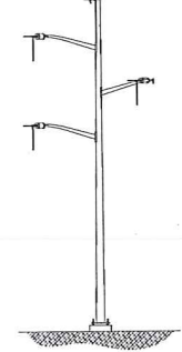
115_ST_DADE_SS STEEL DAVIT ARM DEAD END-SINGLE STRING DWG. 400298-C-S-15
