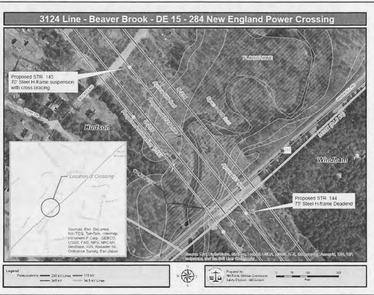
Figure 1: This is the proposed 3124 line shown in the center of the 350 foot ROW. The span of 919 feet crosses both the Beaver Brook and a parcel of the NH DOT. The respective Support structures are 485 feet and 275 feet to the banks of the Beaver Brook. Note also Route 111 is crossed but not subject of this petition. Existing 230 kv lines N214 and O215 are shown as reference. Proposed relocation of Y-151 115 kV is also depicted.
