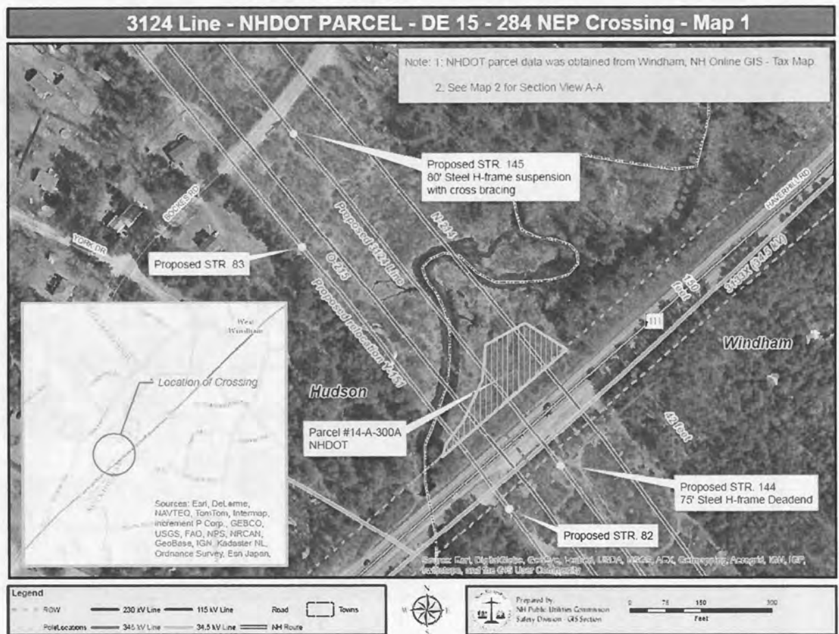
Figure 2: 345kV, designated as the 3124 Line, a span of approximately 919 feet in Windham and Hudson, NH. The yellow highlighted parcel is the public land owned by NH DOT that the petition seeks to cross. This is outside of the Highway ROW thus RSA 231:161 does not apply. RSA 371:17 does apply. Note this crossing is referenced as Crossing #2 in this Staff Memorandum. Cross Section A-A is shown on Appendix A – Figure 3
