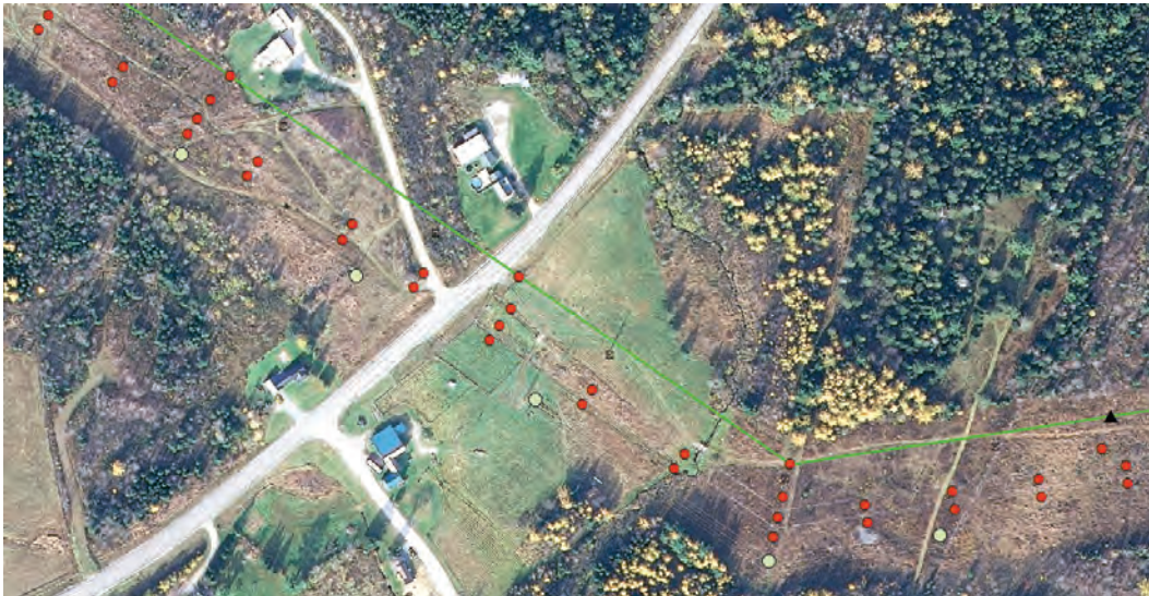
Figure 24. Aerial view of the Project as it crosses Route 116 in Whitefield. The green line represents the centerline of HVDC structures, red dots represent proposed monopole structures, and the light green dots represent existing 115 kV structures to remain. While the proposed structures maintain a similar spacing rhythm, this does not match the existing line that will remain, and places a 90' HVDC structure within 40' of the roadway.
