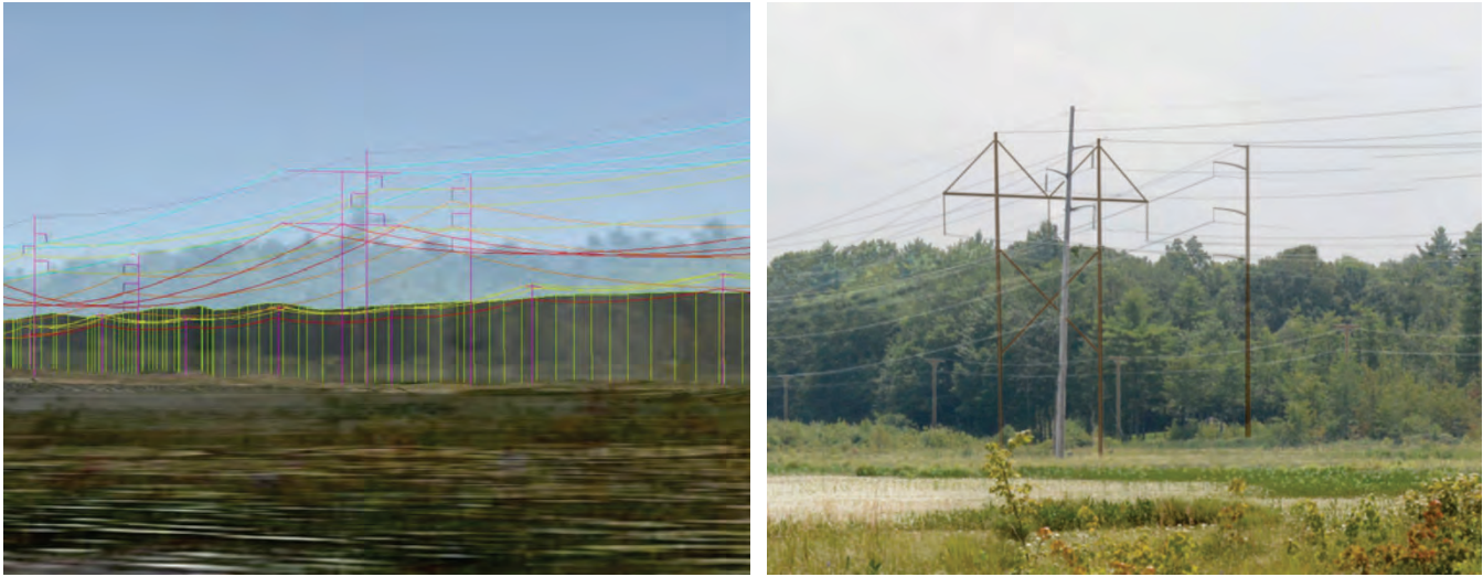
Figure 14. Left: A cropped and enlarged image from Google Earth Pro depicting the proposed three-pole structure. The KMZ used in Google Earth Pro does not include obvious information identifying this as a three-pole structure. Right: The photosimulation provided in the NPT VIA. The source for the weathering steel material used in the DeWan & Associates simulation is unknown.
