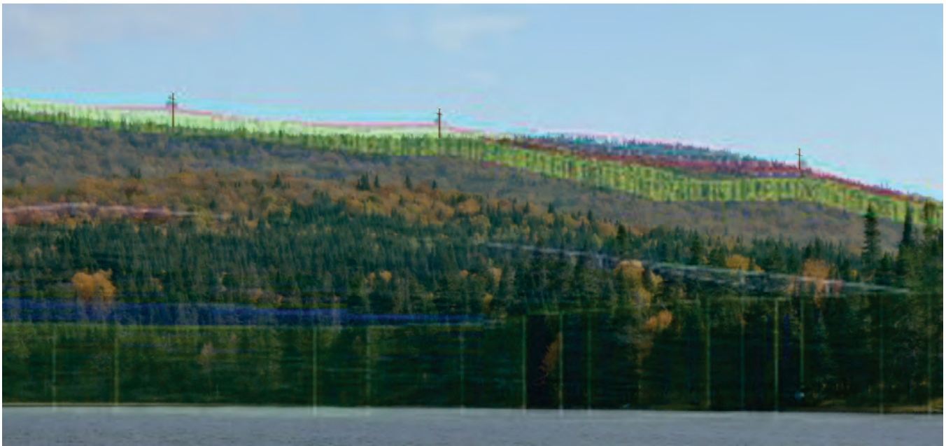
Figure 18. A cropped and enlarged image from the Photoshop panorama file used to create the photosimulation depicting the KMZ image overlaid on the panorama image. The structures are not placed to exactly match the heights as indicated by the KMZ image export.
