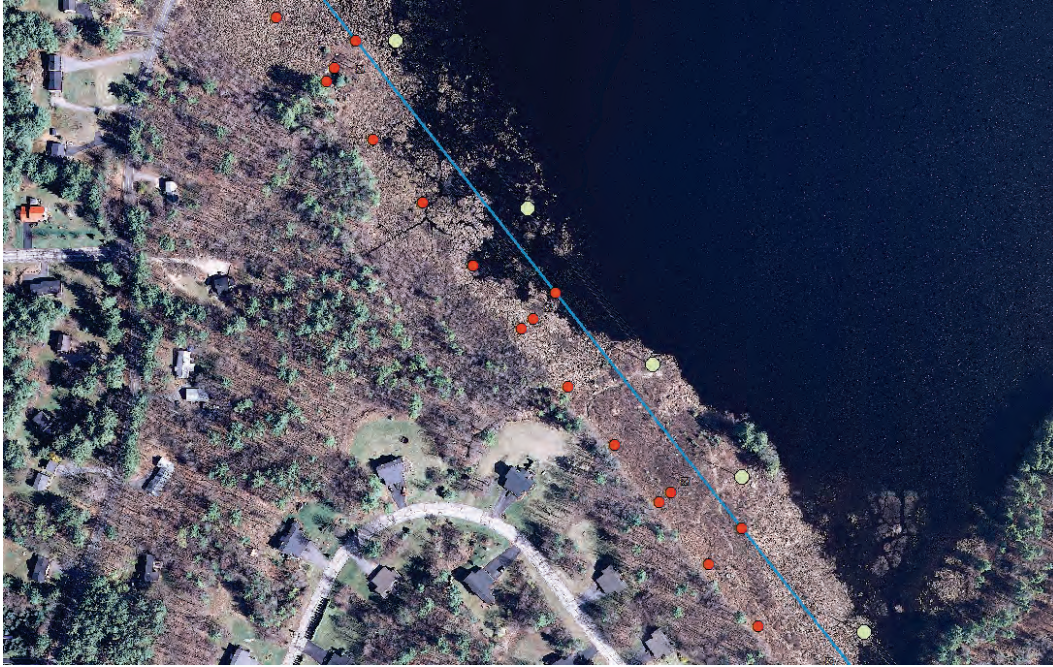
Figure 27. Aerial view of the proposed project as it crosses Turtle Pond. The blue line represents the 345 kV centerline, red dots represent proposed monopole structures, and light green dots represent existing 115 kV structures to remain. The proposed structures do not maintain a similar spacing rhythm, and do not match the existing line that will remain. A review of the simulation in the NPT VIA at 5-19 and 5-21 also does not reveal a consistent spacing of the proposed structures compared with the existing structures.
