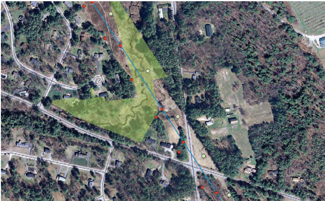
Figure 26. Aerial view of the proposed project as it crosses Hoit Road and Route 132 (Mountain Road) in Concord. The blue line represents the 345 kV centerline, red dots represent proposed monopole structures, and light green dots represent existing 115 kV structures to remain. The proposed structures do not maintain a similar spacing rhythm, and do not match the existing line that will remain, and a new 90' 345 kV structure is placed within 40' of the roadway. The green shaded area is the Brookwood Open Space, part of the New Hampshire Conservation/Public Lands dataset. Both roads are part of the Canterbury Shaker Village Byway and are heavily traveled by motorists and bicycle riders experiencing their scenic quality.
