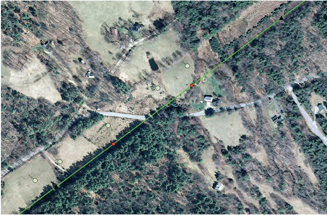
Figure 25. Aerial view of the proposed project as it crosses Peaked Hill Road in Bristol. The green line represents the centerline of the HVDC structures, red dots represent proposed monopole structures, and the light green dots represent existing 115 kV structures to remain. The HVDC spacing does not match the existing structures.
