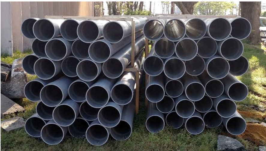
Figure 18: Example of 8 inch PVC duct bank.
