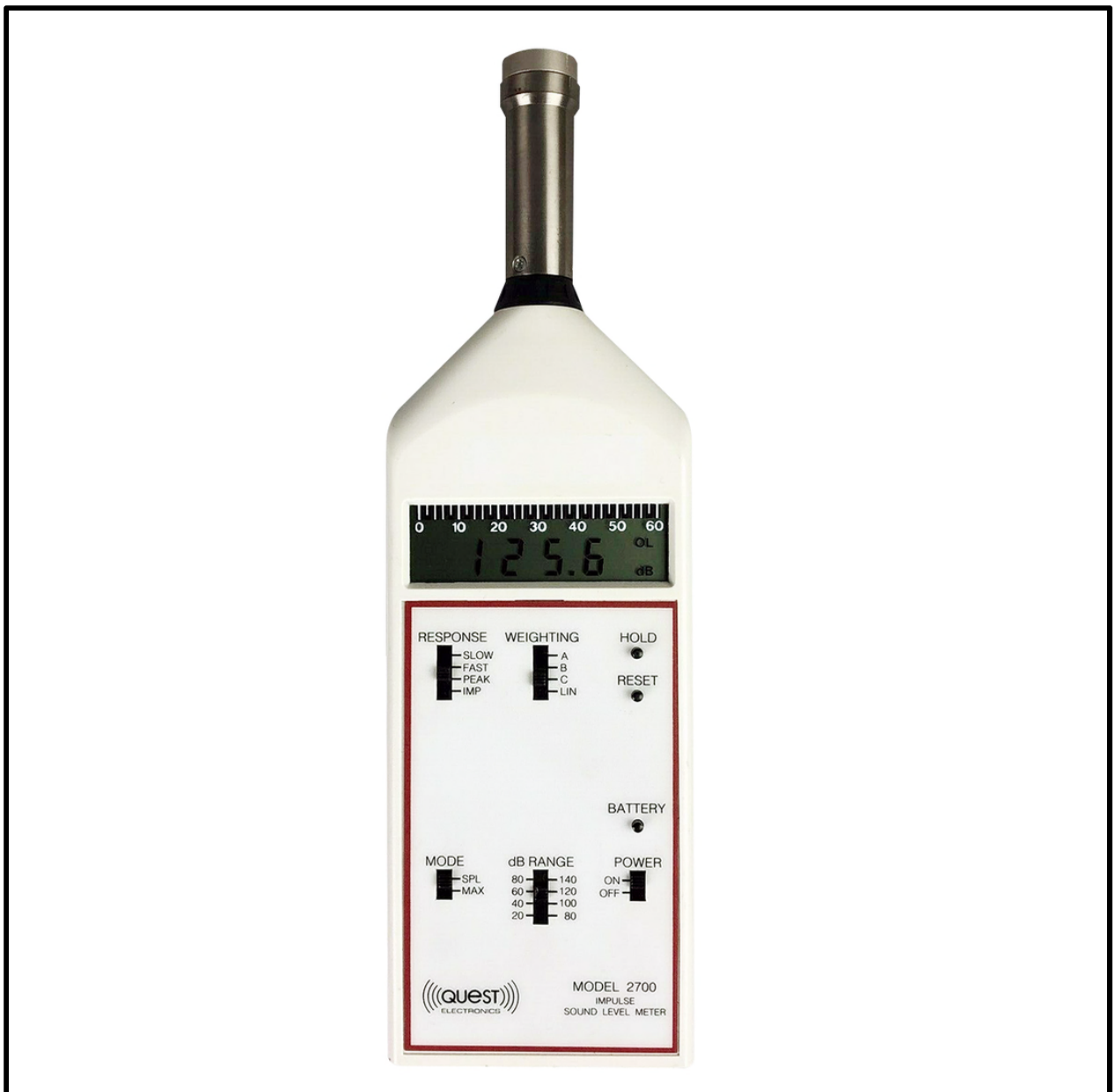
Figure 3. Sound Level Meter with Fast/Slow Response Setting
