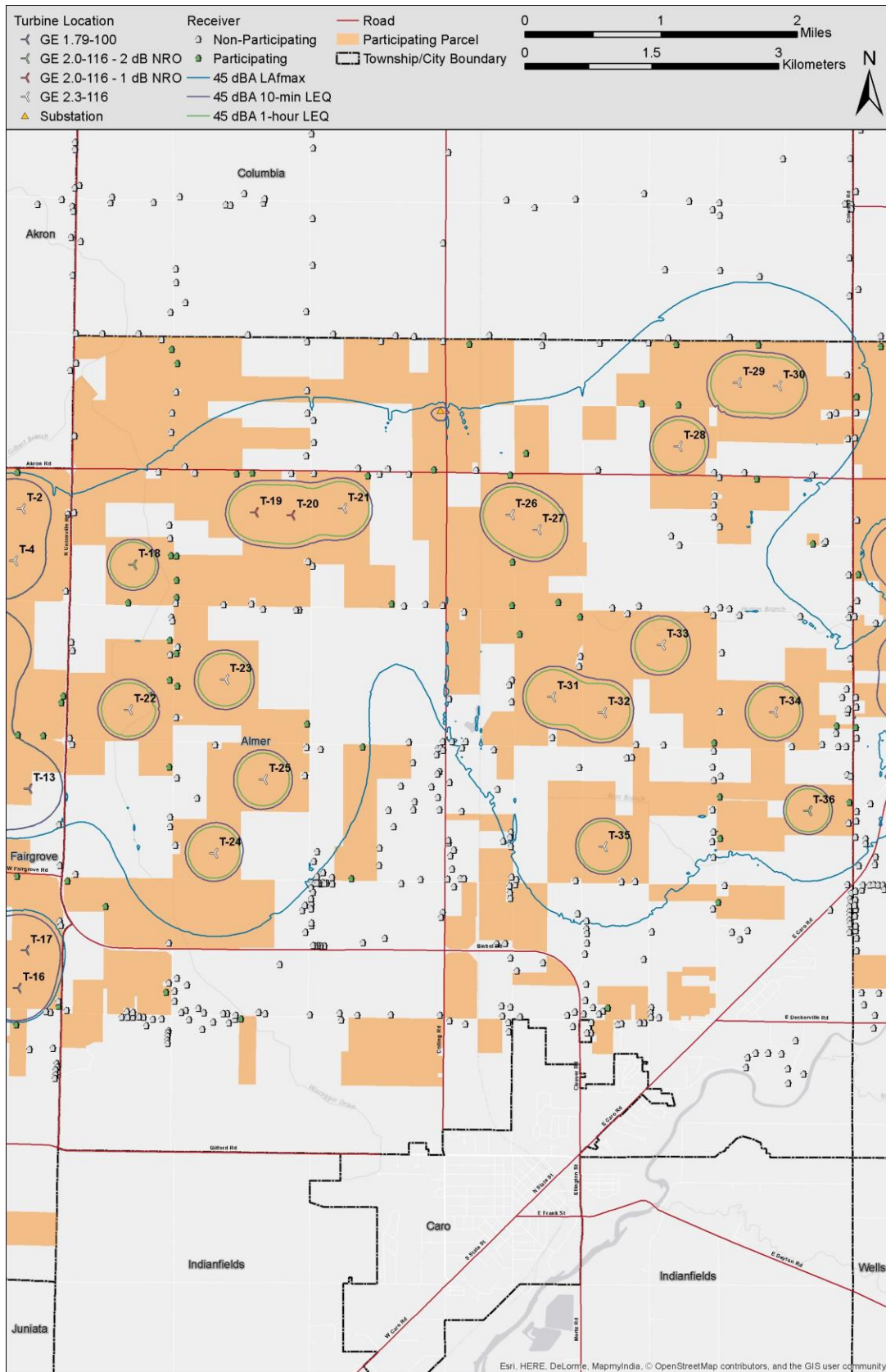
FIGURE 1: 45 dBA ISOLINES FOR MAXIMUM 1-HOUR L Eq , 10-MINUTE L Eq , AND L Fmax
